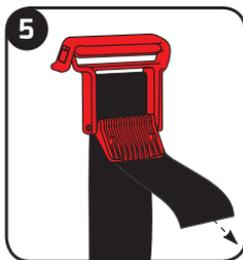
To shorten or lengthen the shoulder belt guide pull the strap in the desired direction.
