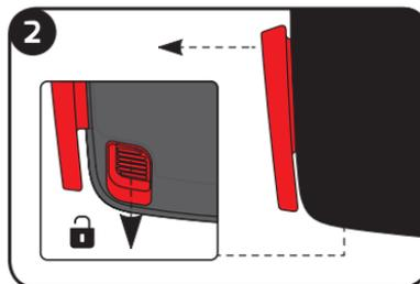
To unlock the lap belt guides, slide the Lap Belt Guide Release button forward.
