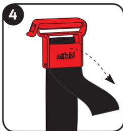
To access the shoulder belt guide strap, pull open the shoulder belt guide buckle.
