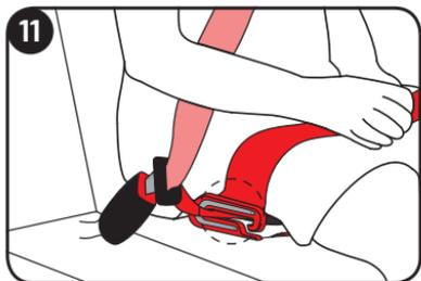
Insert the lap portion only of the vehicle seat belt through the red belt guides on each side of the booster.
