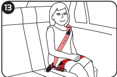
Remove any twists or seat belt slack by pulling on the lap portion and then the diagonal portion of the adult seat belt. Ensure that the lap portion is positioned over the child's lap and supported on the child's pelvis.
