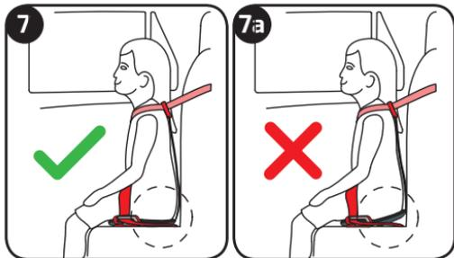
Ensure that the booster seat is laid flat and up against the back rest of the vehicle seat.
