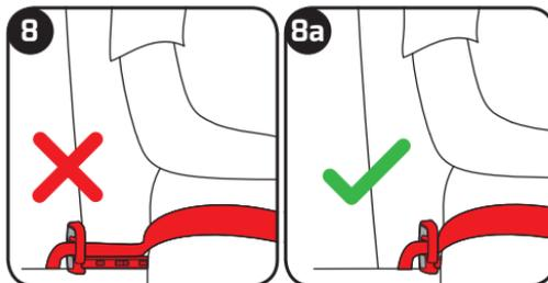
Position your child sitting upright on the booster seat and if necessary, slide lap belt guides into the position nearest to, but not touching the child's thigh. Pull out on lap belt guides to check they are locked into position.
