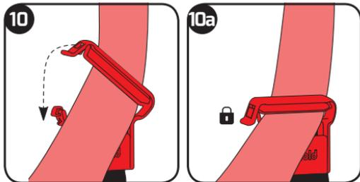
To position the shoulder belt guide, attach the shoulder belt guide to the diagonal portion of the vehicle seat belt, by opening the clip and inserting the seat belt. Then close the clip.
