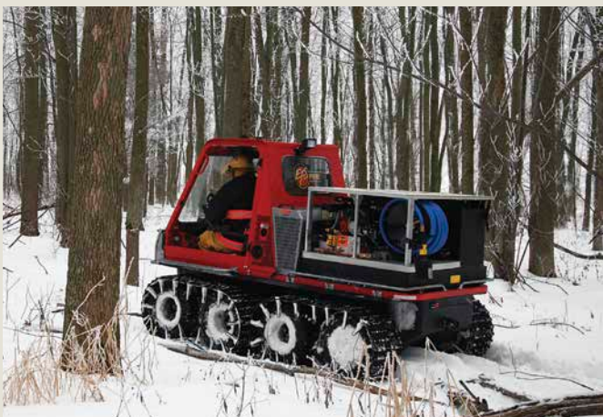
ARGO 8x8 Centaur Fire Chief with CET 80 gallon tank, foam system, fire pump and storage compartments.
