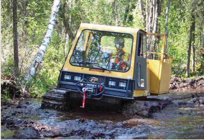
ARGO 8x8 Centaur with custom cargo box to transport core samples in challenging terrain.
