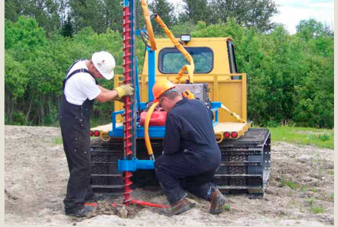
ARGO 8x8 Centaur with Multi-Power drilling system for soil sampling.
