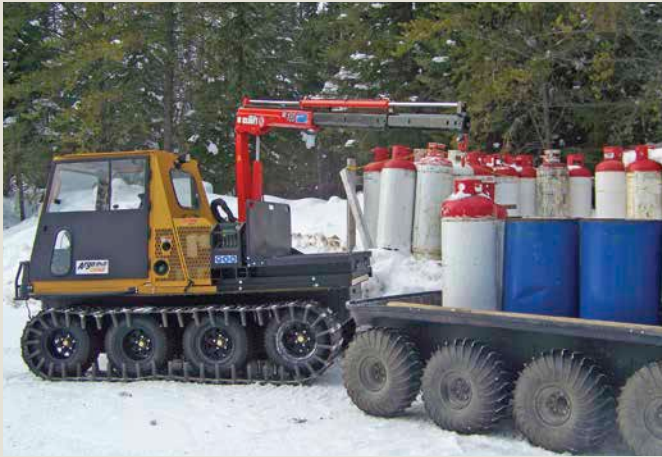
ARGO 8x8 Centaur equipped with Maxilift crane and flat bed pulling 8 wheel trailer.
