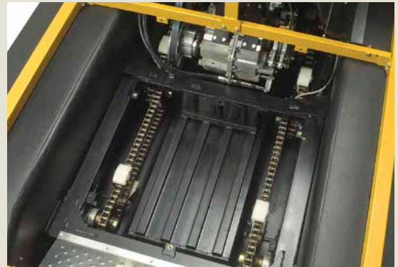
3" (76 mm) tubular frame, strong RC 80 chains with automatic, reversible chain adjusters.
