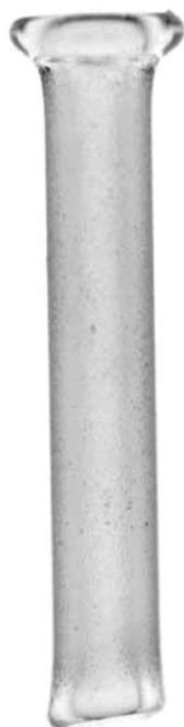
**FIG. 2.** Frosted Jones Pyrex tube, with a collar and angled tip.
