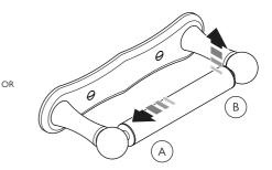
I The paper holder bar is spring loaded at one end. Gently move the paper holder bar to one side (A). Lift the opposite end clear of the support arms (B).
