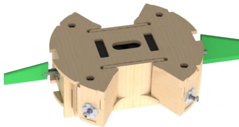
Figure 5: Assembled view of canard housing
