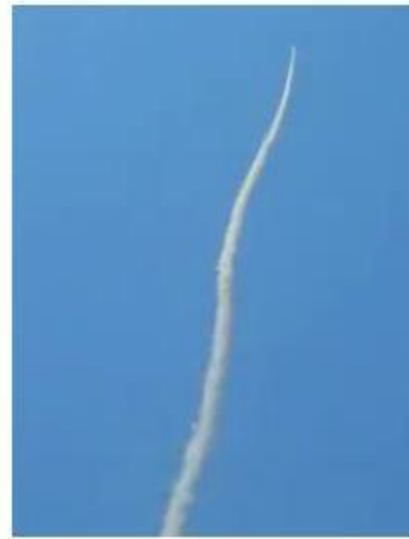
Figure 1: 2015 flight of MASA rocket with dynamic instability
