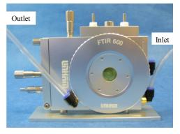
**DSC600 Thermatica** Optical Thermal Analysis Stage
