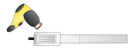
**12.** Connection is now complete. Allow any additional silicone to squeeze out, and wipe off the excess.
