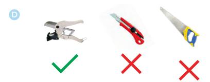
**CUTTING**: Use a PVC cutting device to cut the strip light. Utility knives and/or a saw create uneven and tilted edges, and water damage may occur.
