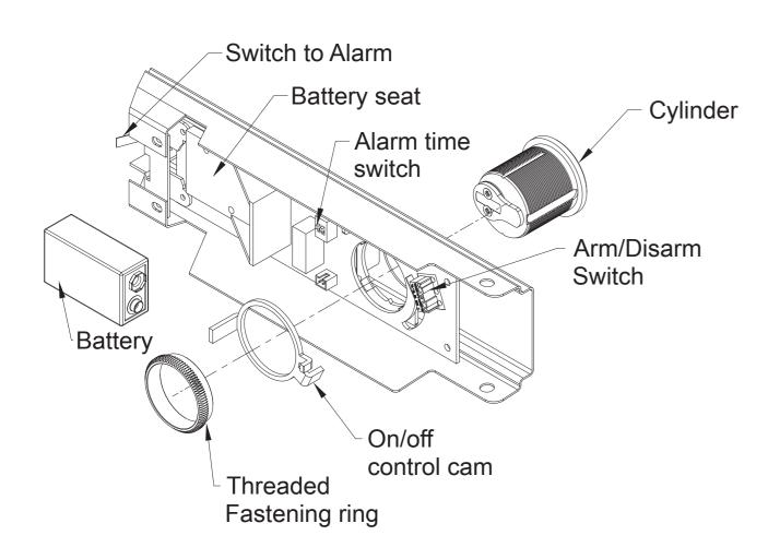
2. Place the 9V Battery onto the panel.
