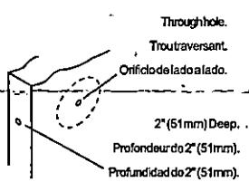
C. Drill the 2-1/8" (54mm) hole about halfway through door, then finish drilling from the other side to prevent splintering.
