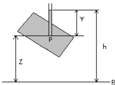
The total potential,  $h$  or head, at the measurement point,  $P$ , which is the open end of the piezometer or the screened interval of the well, consists of  $\Psi$ , the pressure head plus  $Z$ , the elevation head,
