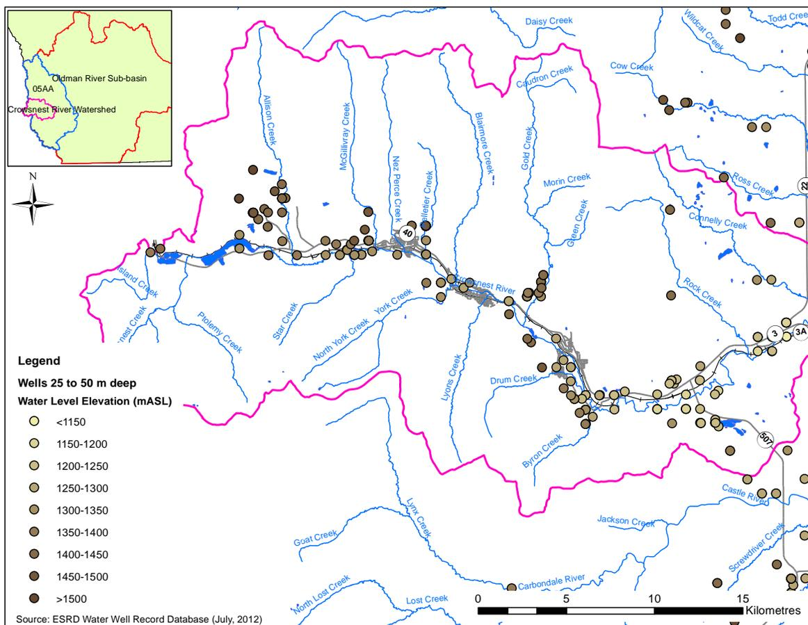
Figure 21 Water level elevations for wells 25 – 50 m Deep
