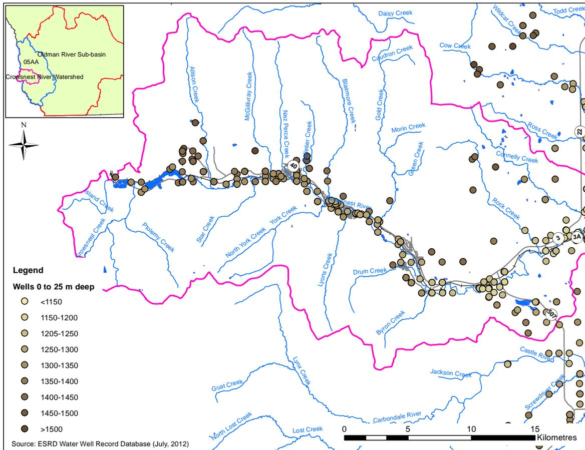
Figure 20 Water level elevations for wells 0 – 25 m Deep
