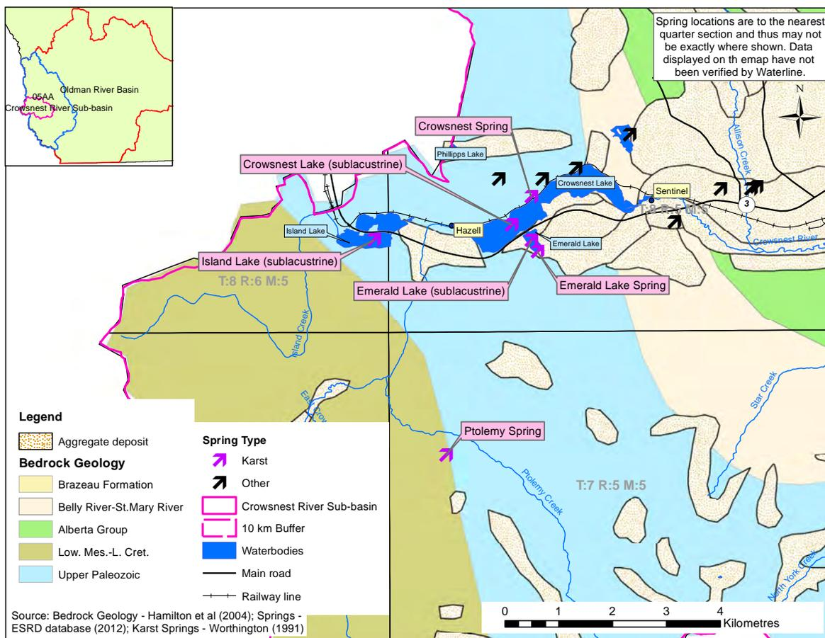
Figure 26 High Volume Discharge Springs
