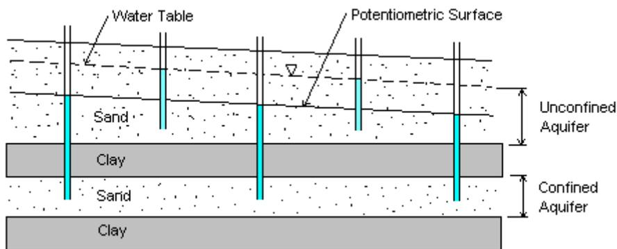
The water table is a potentiometric surface with zero pressure head; the total head consists of elevation head. To be sure that you are monitoring the water table level – the fluid level in the well must be in the screened interval. For a confined aquifer the head may lie within the aquifer or above it – this is not the same as the water table.
