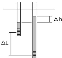
The direction of the vertical gradient (up or down) indicates whether there are local discharge or recharge conditions. The figure below (on the left) shows a water level in the deeper well that is higher than that in the shallow well, indicating an upward gradient exists, this suggests that discharge conditions could exist locally.
