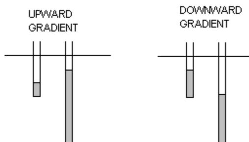
An upward gradient would be expected in areas such as valley floors, at the base of hills or near bodies of water. Downward gradients (the level in the deeper well is deeper than that in the shallow well) are indicative of recharge conditions. These conditions generally exist on topographically high areas.
