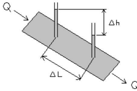
The fluid in the figure above flows from the upper left to the lower right driven by gravity as a result of the difference in elevation between the ends of the sand filled tube. The flow rate is denoted by  $Q$  and has units of  $L^3/T$ . The magnitude of the potential gradient,  $i$ , is the difference in head,  $h$ , between the two manometers divided by the distance,  $L$  between the two manometers.
