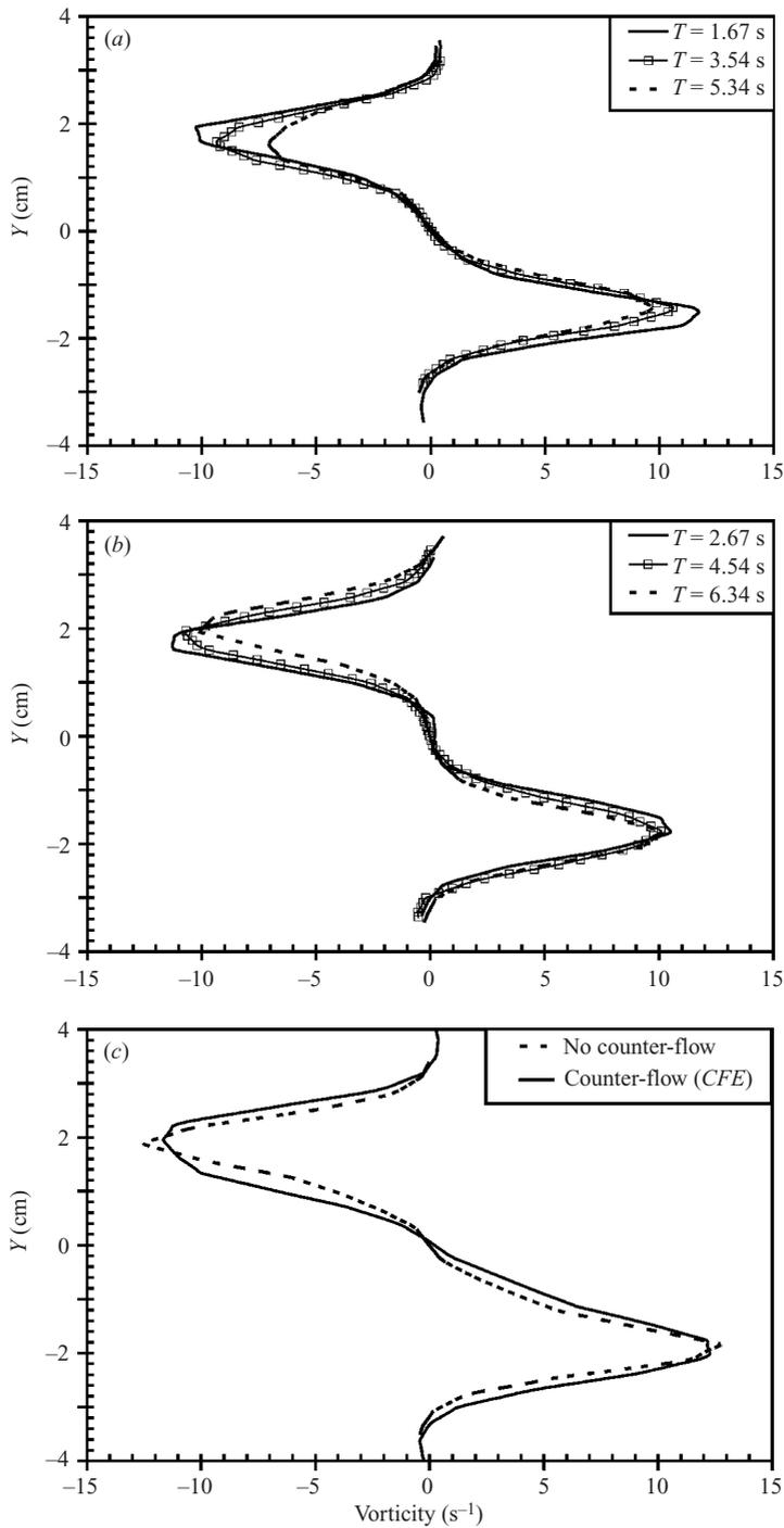
FIGURE 6. (a, b) Temporal evolution of vortex ring vorticity profile for protocols *LD2-CF0* and *LD2-CFE*, respectively; (c) vorticity profiles for protocols *LD4-CF0* and *LD4-CFE* at time  $T = 2.0$  s.
