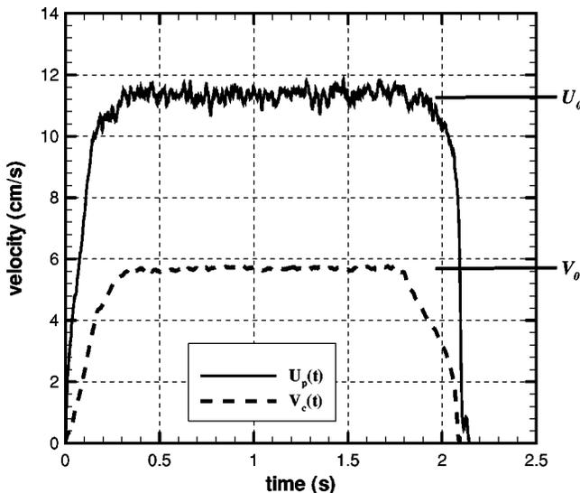
FIG. 2. Piston and co-flow velocity traces for  $R_v = 0.50, U_0 = 11.4 \text{ cm/s}$ . The velocities near shut down ( $t > 1.5 \text{ s}$ ) are not relevant to this study.
