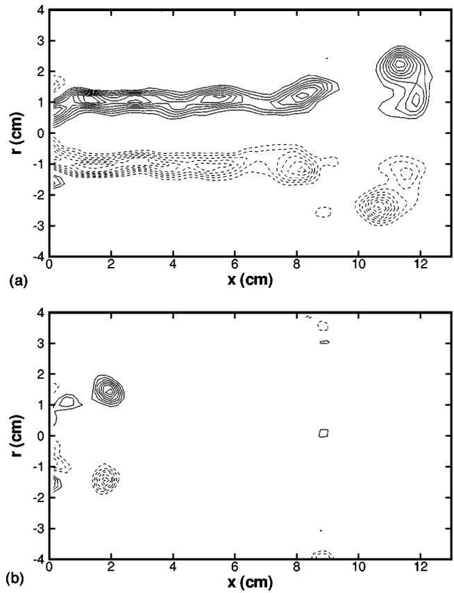
FIG. 4. Vorticity plots at instants just after pinchoff is completed for (a)  $R_v = 0.50$  and (b)  $R_v = 0.75$ , both at  $U_0 = 5.5$  cm/s. The dashed contours represent negative vorticity. The minimum contour plotted of a given sense is  $2 \text{ s}^{-1}$ .
