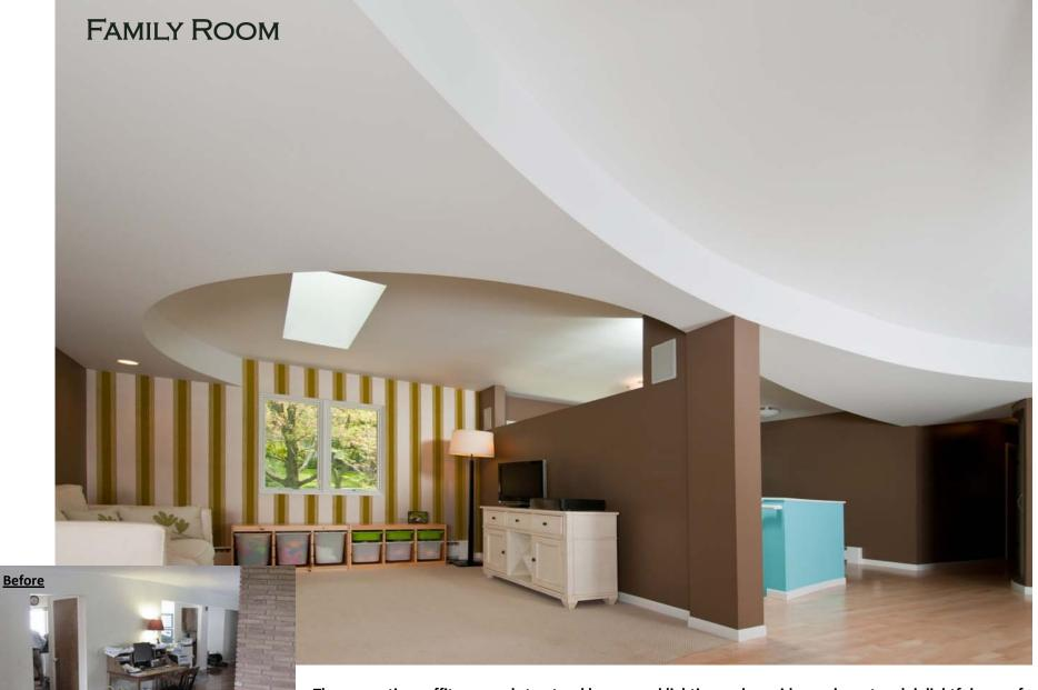
The serpentine soffits conceal structural beams and lighting and provide an elegant and delightful way of connecting separate spaces together. The main path from the bedroom wing to the kitchen follows the dominant curve.
