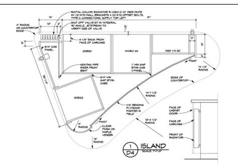
The island,  $9' \times 6'$ , required precision in fabrication to fit all the desired cabinetry, the hot water radiator, the curved veneers, and to align with the room. Cabinetry parts were cut on our CNC router based on our detailed drawings.
