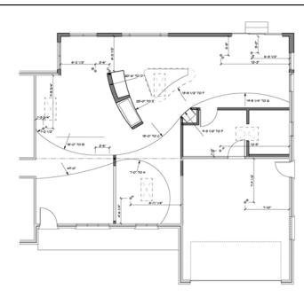
All curves were laid out on our CAD drawings. Top and bottom plates for the curved walls and soffits were then cut on our CNC router machine for ease and accuracy as many layout points for the curves were outside of the building.
