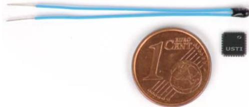
Figure 7. Thermistors S861 (EPCOS) and USTI IC in 5x5 mm MLF package - main components of temperature sensing systems.
