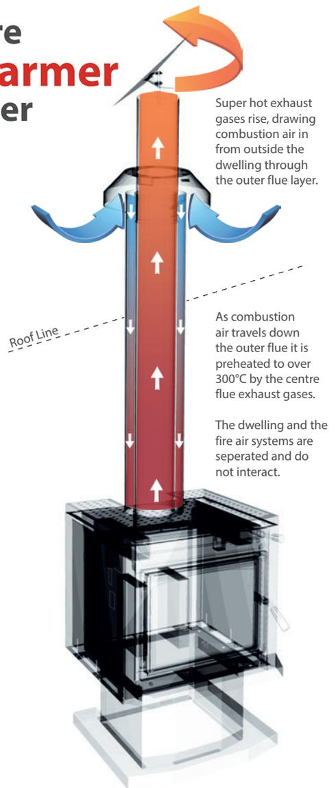
Combustion air is drawn from outside the home, down the outer section of the flue system.
