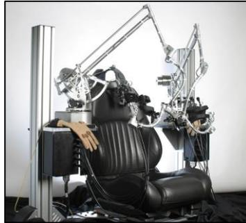
Figure 1: Haptic Workstation
