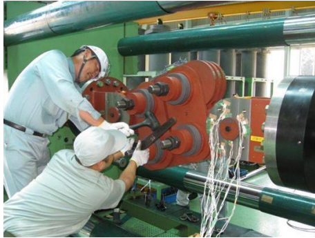
Figure 27 - Test setup of 1500 kN damper in testing facilities in Japan
