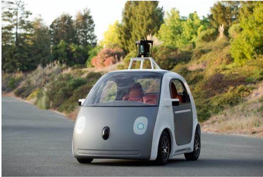
Over and above the new innovative LiDAR systems for AVs, real-time speed and distance of vehicles is determined using wheel speed sensors, front/rear mounted radar and a pair of cameras with overlapping fields of view on each end for tracking real-time distances in 'stereo.'
