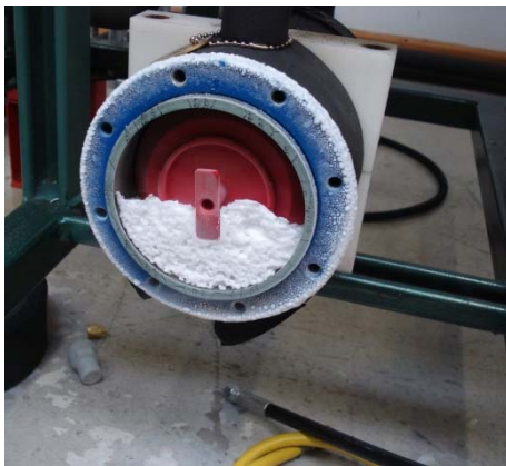
Figure 16, example of dry ice and moisture within a drier core housing
