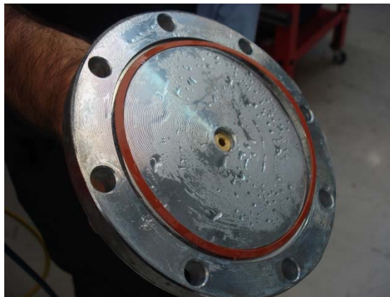
Figure 16, example of dry ice and moisture within a drier core housing
