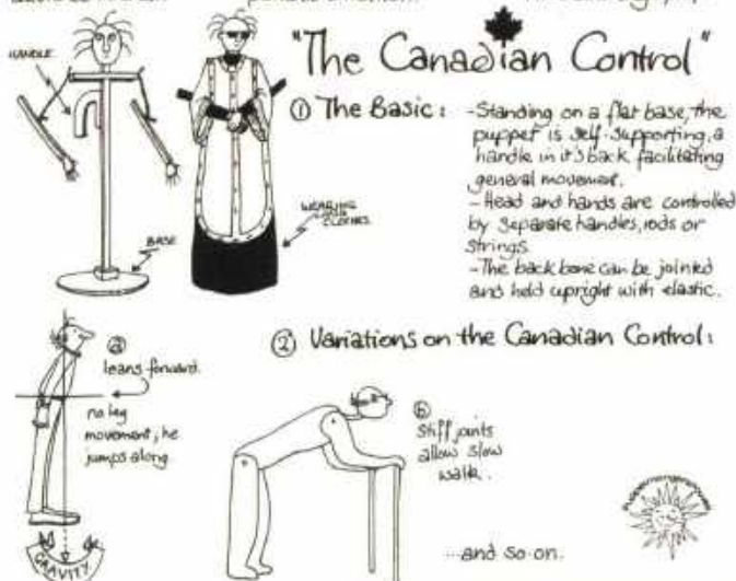
INFORMATION SHEET ON THE "CANADIAN CONTROL" CREATED BY THE POWELLS, ILLUSTRATIONS BY ANN POWELL
