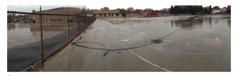
(Parkside School for the Arts) Picture of a typical Milwaukee area school playground, originally installed to reduce maintenance costs, but has resulted in increased stormwater runoff - increasing the instances of combined sewer overflows and impaired water bodies and has reduced green space for students, reducing play, outdoor eco-literacy opportunities, and educational outcomes
