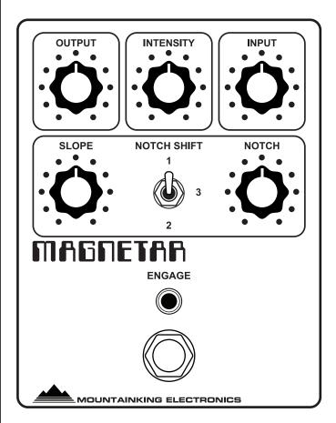
**INPUT:** This controls the strength of the signal going into the pedal. It affects the sensitivity of the gating and also influences the texture and saturation of the fuzz, especially when the INTENSITY control is at lower settings.
