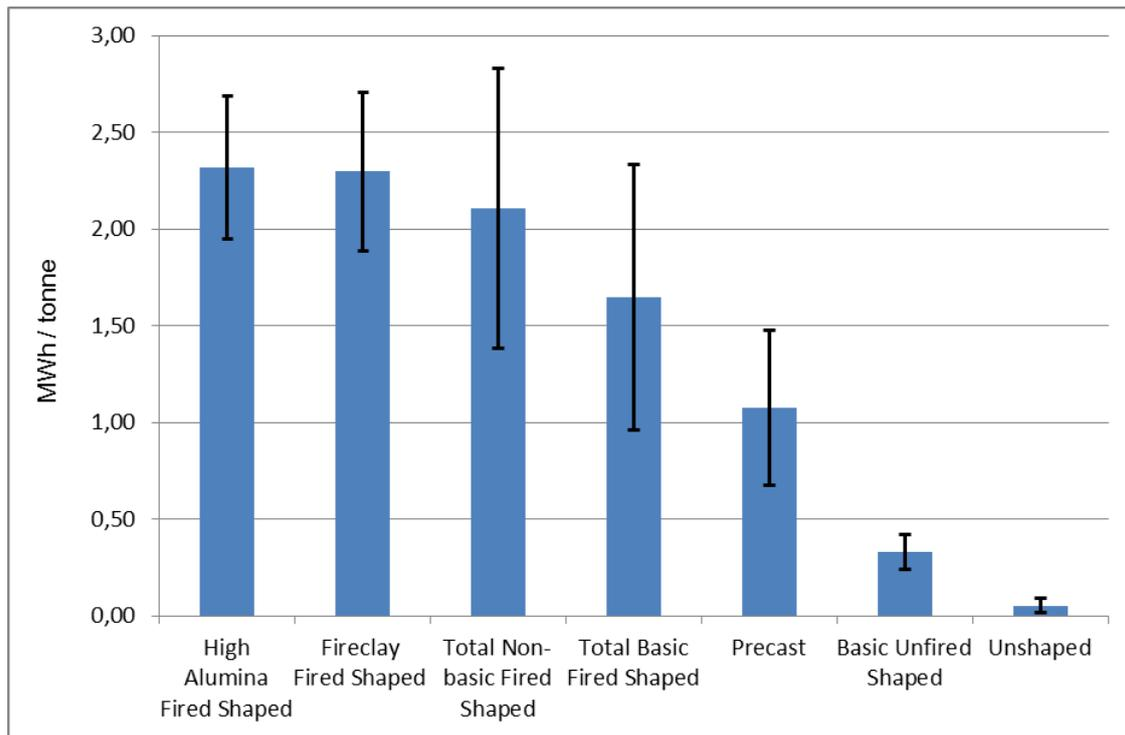
Fig. 5: Energy intensity of different refractory product groups
