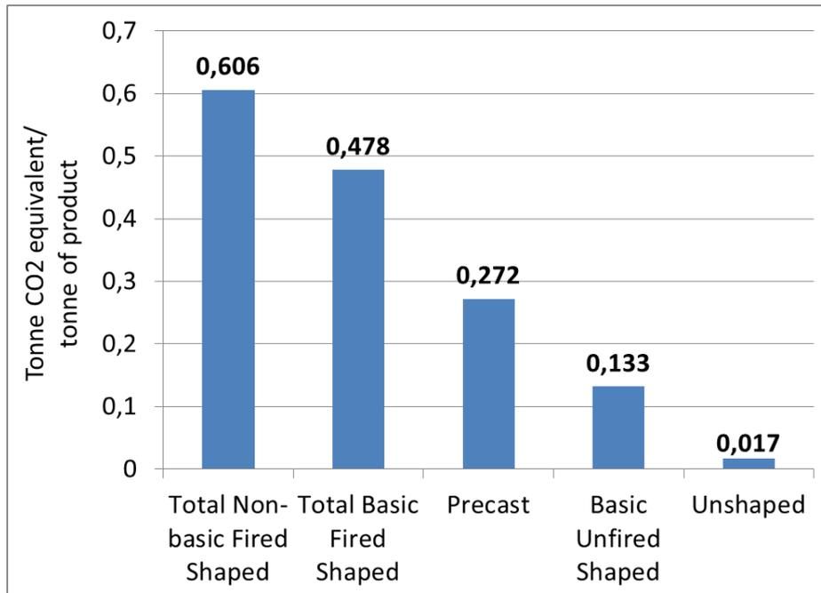
*Fig. 6: Product carbon footprint of different refractory product groups*
