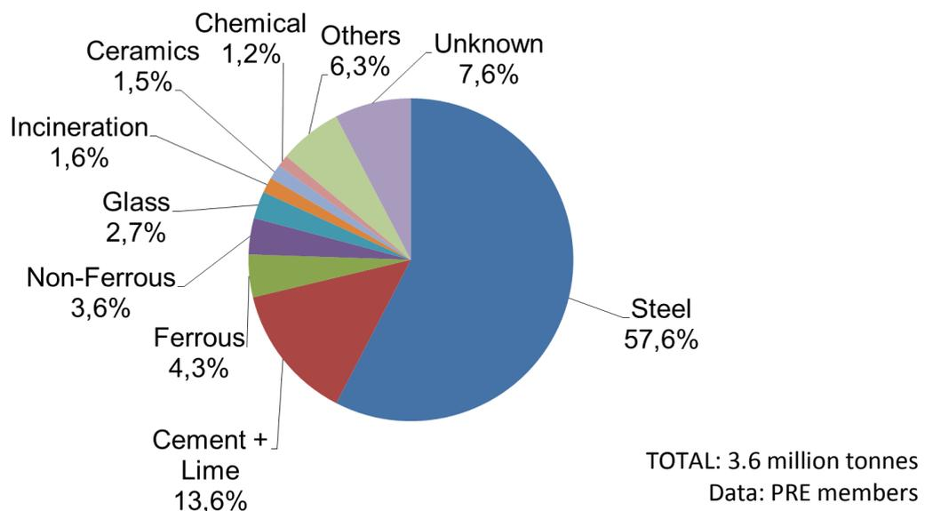
Fig. 2: End-use applications of refractory products
