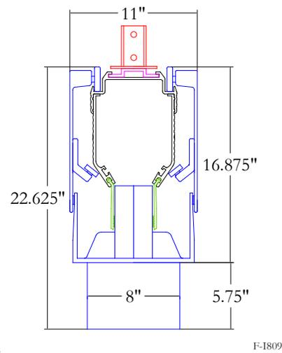
Dimensions are given for the rubber seals, exterior coupling, and suspension bracket adapter. All dimensions are in inches, rounded to the nearest 1/8".
