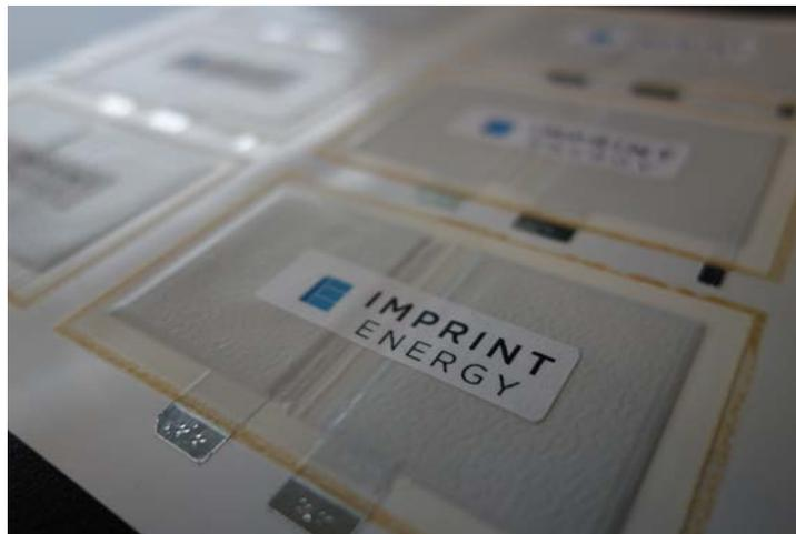
*Above: An Imprint Energy ultrathin battery, designed to power IoT devices using Semtech’s LoRa® technology.*
