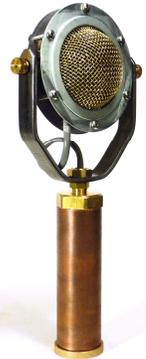
The capsule is a Chinese-made electret condenser individually tested and selected – roughly 30% of capsules are rejected for not meeting design criteria. The circuit is a transformerless FET with fully balanced output and EMI noise suppression. Other electrical components in the signal path are highest quality metal film resistors, polypropylene and polystyrene capacitors, and individually tested, hand-matched and biased transistors and JFETs.
