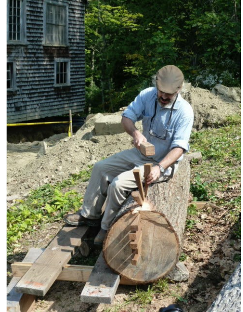
MHHA board member Wade Smith (Mill Hollow Works) demonstrates the art of riving or splitting logs for fences. Photo: Tafi Brown
