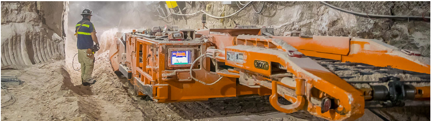
Crews use a continuous miner to level the floor near the Salt Shaft. Due to the natural movement of salt, maintenance and ground control personnel are constantly working to maintain the underground facilities while on the surface, crews work to update and maintain the infrastructure of the nation's only deep geological repository.
