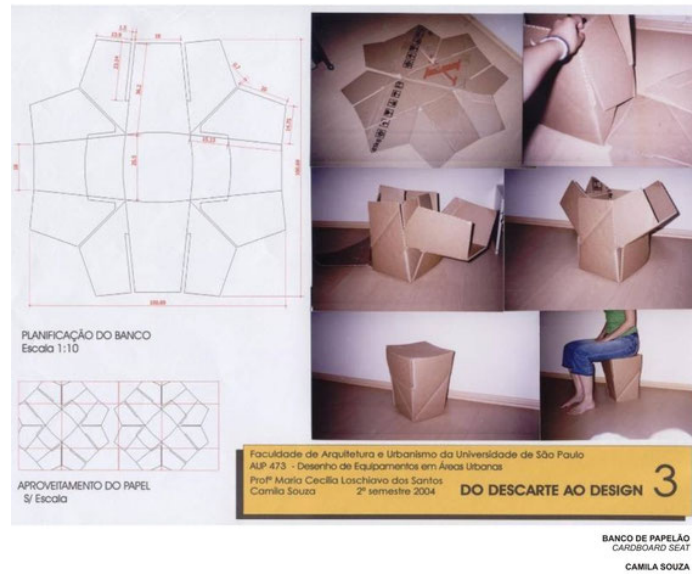
Figure 5 Cardboard Bench made from folds and cuts in the material. Student: Camila Souza. Year: 2004.
