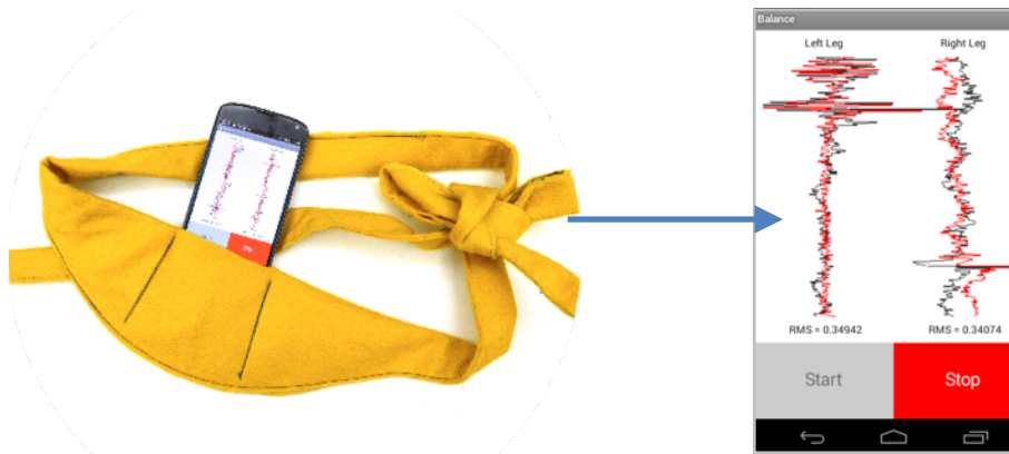
Figure 15: Quantitative testing version of the application, L to R, phone application and belt, zoomed in view of interface
