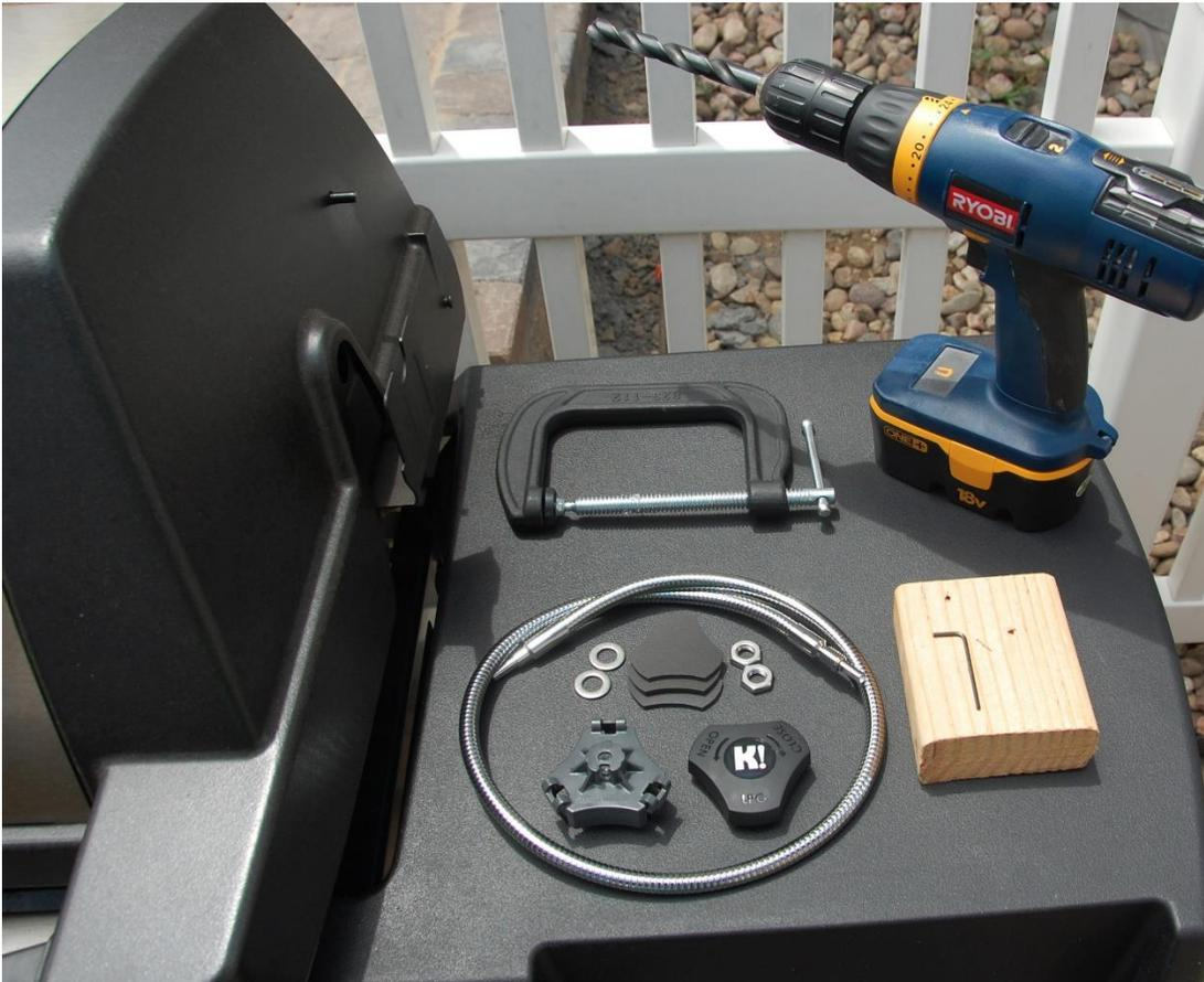
1. Think about where you want to mount the user knob. In this method, the user knob will be mounted by drilling a hole in your grill's control panel or other location. **CAUTION: be sure to check for obstructions behind your drill site such as gas lines, electronic ignition wires, etc.** Additionally, pay attention to where you will route the flexible shaft. Make sure the shaft won't interfere with any of your grill's other functions, such as closing the doors.
