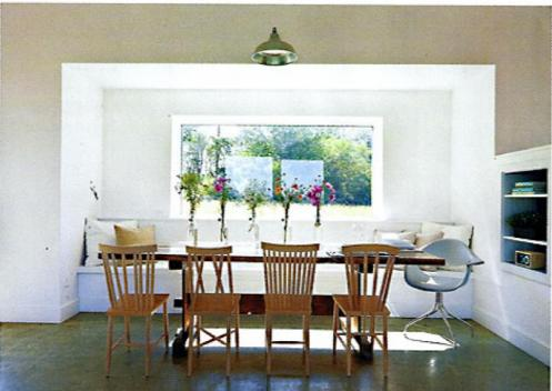
HARNESS THE SUN To save on heating costs, Horowitz installed oversize triple-pane, high-solargain Schuco windows on the southern side of the house, inviting solar rays deep into the abode and allowing the sun to warm the concrete floor throughout the day. Smaller north-facing windows offer views of the surrounding farmland.
