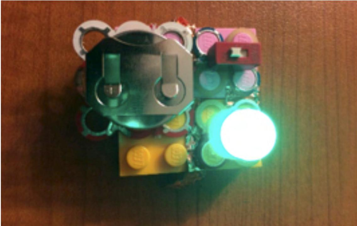
your design, or even put it inside, it can shake the whole structure. In the top photos, a tiny circuit was assembled using copper tape on LEGO bricks. Try adding a motor and putting the circuit into a paper box to make a moving creature! You can also embed the circuits on a cork, pins and pipe cleaners. Take a look at the [www.lectrify.it/projects](http://www.lectrify.it/projects) for more ideas!
