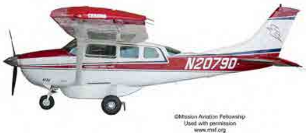
Figure 1.4.1 Showing side view of Aerocet Cargo Pod on Cessna 206 Aircraft.
