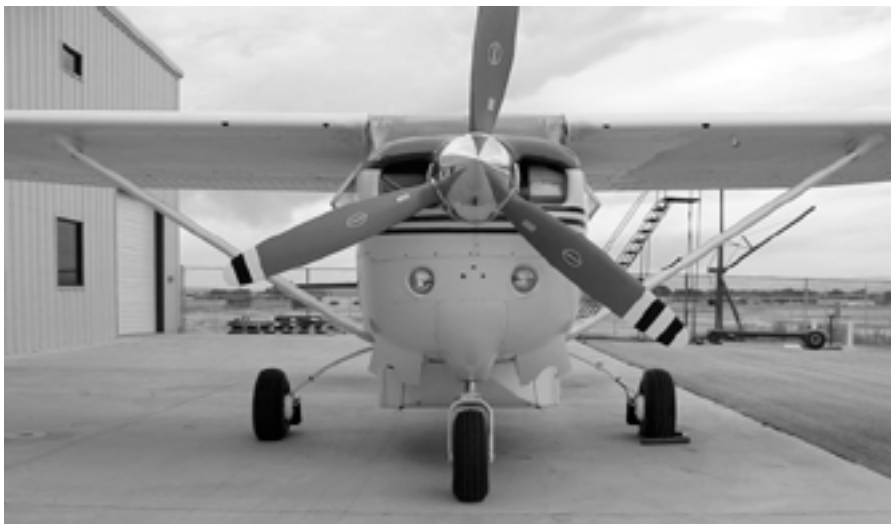
Figure 1.4.2 Showing front view of Aerocet Cargo Pod on Cessna 206 Aircraft.
