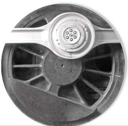
Big and small - The Class J features 70" drivers and the 3460-Class 84" drivers.
