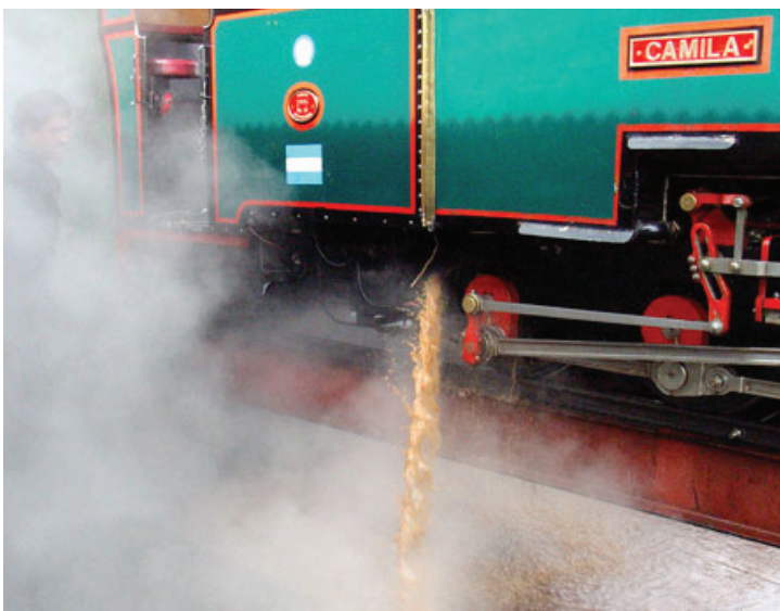
Step 1: Drain the Boiler Washout plugs are opened on the top of the boiler to vent and on the bottom of the boiler to drain out the initial boiler water in the system.
