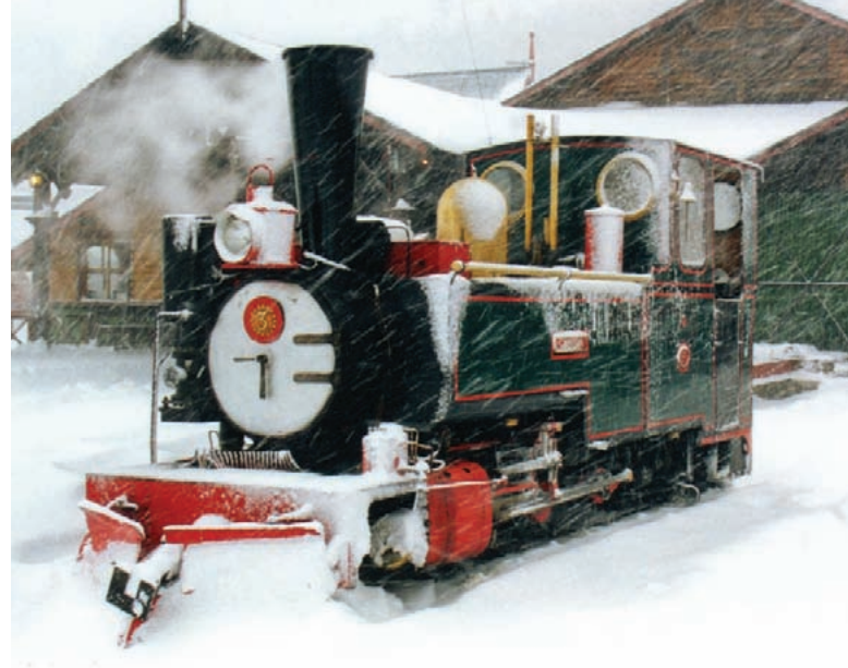
Rain, sleet, or snow , the trains must run. This image shows locomotive 3, ‘Camila,’ when in service on the railway post-rebuild and Stage 1 modification. Note the stack profile indicative of an advanced exhaust.
