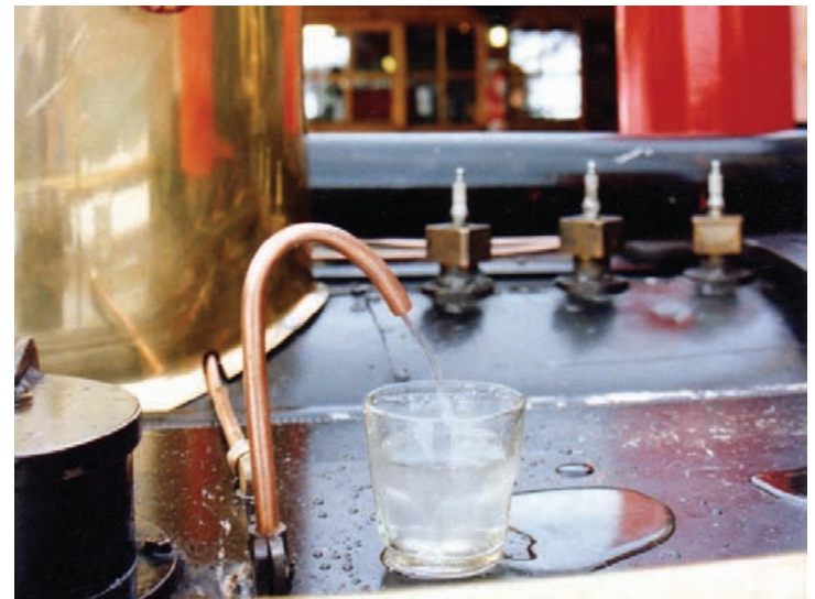
Despite the brown water, pure steam is generated in the boiler for propulsion. This take-off spout pulls steam from the dome and is used for purity trials. Compare the color of this water to that on PAGES 12 and 13.
