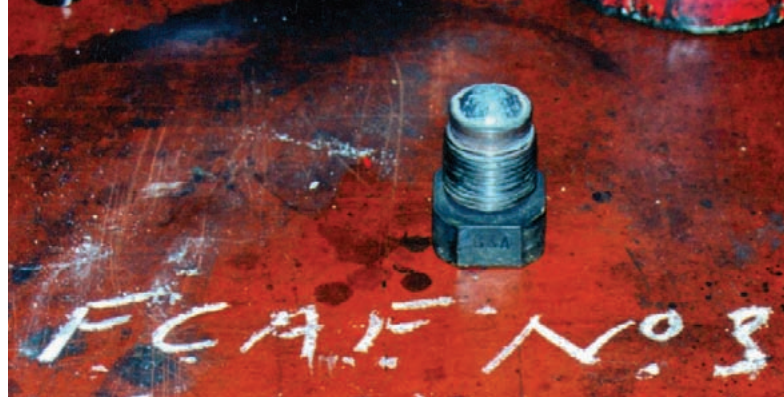
This diagram and photo show the fundamentals of the fusible plugs. The diagram at LEFT shows three types of plugs. In each case, a core of lead alloy is cast such that, in the case of low water, that core melts prior to the softening of the sheets, causing water to pour onto the fire and put it out. The image at right shows the plug from FCAF No. 3. Note the different metal in the core of the plug
