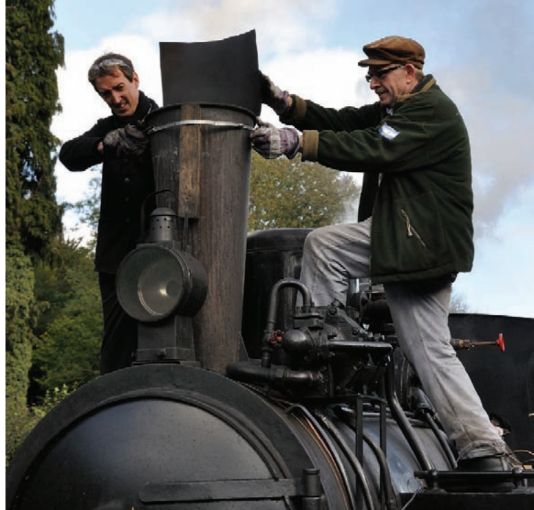
The Author, at RIGHT, is shown affixing a test apparatus to a locomotive during steam purity trials on the WELSHPOOL & LLANFAIR LIGHT RAILWAY in 2012.
