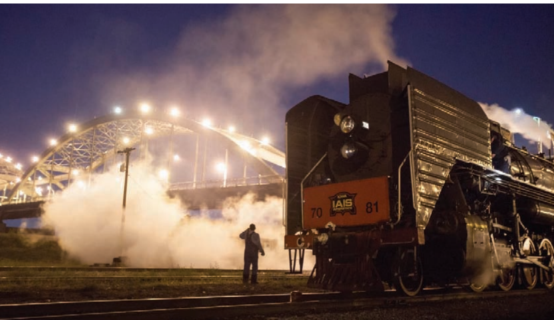
Often quite dramatic, blowing down the boiler removes sediment from the lowest reaches of the system, where it tends to settle. This image shows Iowa Interstate QJ locomotive 7081 blowing down its boiler in Rock Island, Illinois on July 29, 2011. Photograph by Scott Lothes and courtesy of the Center for Railroad Photography and Art - railphoto-art.org.
