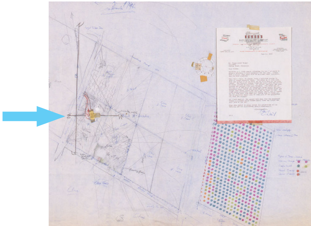
Schematic Site Plan of Lot 8 drawn by Frank Lloyd Wright in 1950; arrow indicates location of the David Wright House. Note the ripples drawn in pencil by Frank Lloyd Wright on Lot 4 to the north, indicating that citrus orchard was part of design concept. Color coded drawing at right was made by David of Lot 7, identifying all the trees and their condition; when he concluded that too many trees would be lost if he built there, he bought Lot 8 to the west (a parcel with far fewer trees). (Sketch: FLLW FDN # 5030.011)
