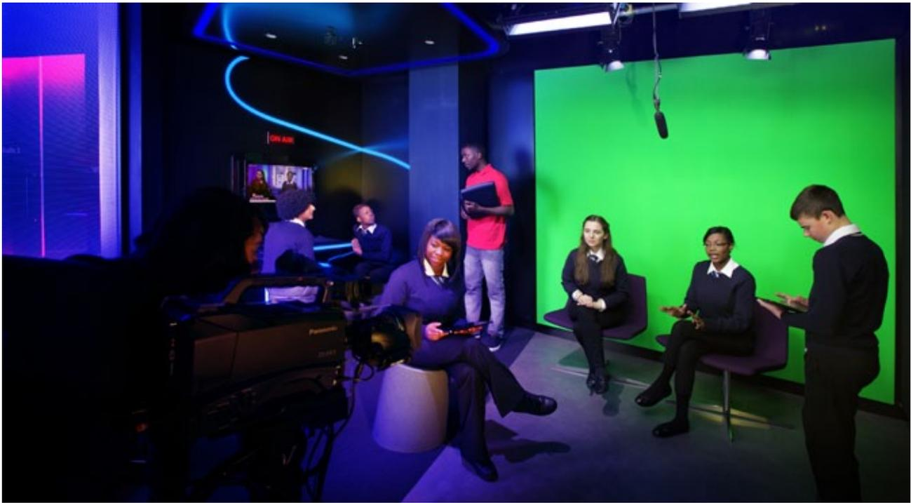
Architectural feature lighting includes RGB LED strips set into the walls, control desks and floating ceilings above the individual interactive edit suites. General task lighting to the edit suites comes from recessed LED down lights set into suspended panels.
