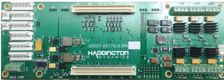
The board measures 16.5cm by 5.7cm, the FPGA board sits on top.
