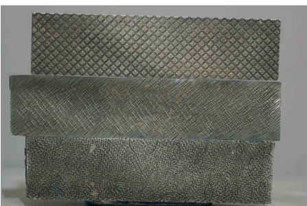
Figure 70 Handmade antique roller die plates like this can serve as matting tool plates.
