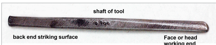
Figure 5 A typical chasing tool with its parts labeled
