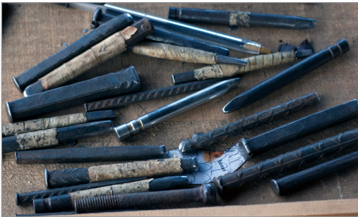
Figure 90 A mixture of Mexican tools made from valve stems, rebar, other punches, etc. The same is done across the world. Note the wrapping of tools to improve the grip.
