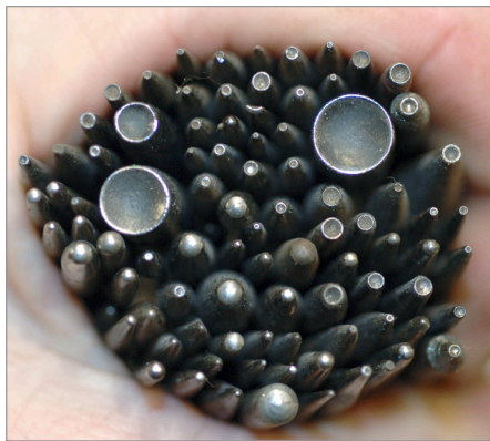
Figure 56 A group of concave and convex pearl punches
