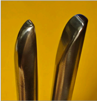
Figure 76 David Huang calls these side tools “round liner” and “flat liner.”
