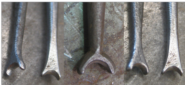
Figure 53 These are Mexican tools for necking in a veined line, creating a series of bumps from the raised line.
