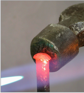
Figure 47 Striking a red-hot tool to upset it
