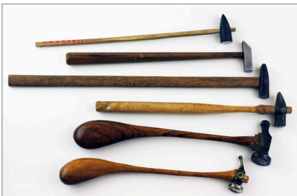
Figure 18 Chasing hammers: The two bottom ones are European; above them in order are Indian, Japanese, Thai and Korean. Note the differences in hammer face size.
