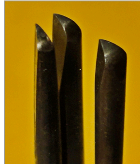
Figure 77 Huang calls these tools “corner tucking” tools.
