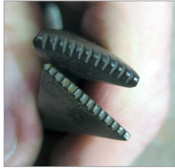
Figure 62 These are Mexican line chain tools, where the end of the tool registers into the last dent of the previous strike.
