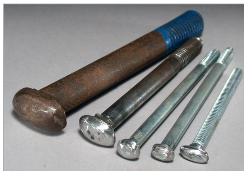
Figure 88 This is a set of forming tools ground out of bolt heads.
