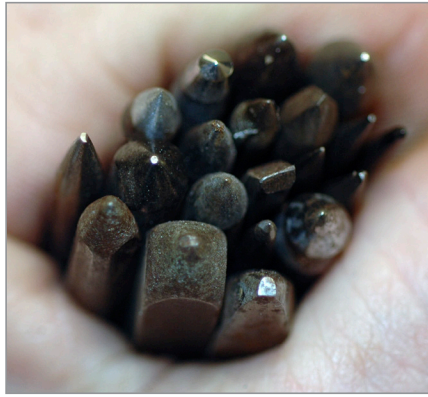
Figure 67 A selection of conical punches
