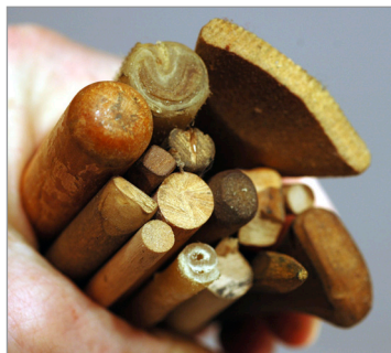
Figure 28 A selection of my soft tools: wood, rawhide, bamboo and plastic
