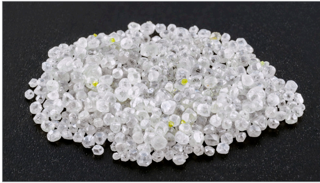
Figure 2 A parcel of approximately 10 carats of HPHT-grown colorless diamond melee produced in China. Each colorless crystal is attached to a yellow synthetic diamond seed on which the crystal is grown. When fashioned as gemstones, each crystal will produce a small (~0.01 carat) round-brilliant cut stone.
