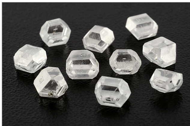
Figure 1 Colorless synthetic diamond crystals grown by the HPHT method in China. The crystals weigh about 2 carats each, and they display the combination of cube and octahedral crystal faces which is characteristic of HPHT-grown material. Photo Jian Xin Liao, ©GIA
