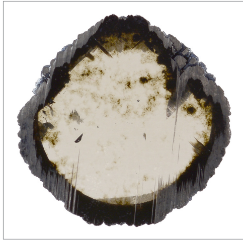
Figure 3 A tabular synthetic diamond crystal grown by the CVD method. Diamond crystals grown by this technique usually exhibit a black outer edge of polycrystalline non-diamond carbon. This dark outer edge is first removed, and the cut gemstone is then fabricated from the central portion of the crystal. This crystal was grown by GIA researchers.
