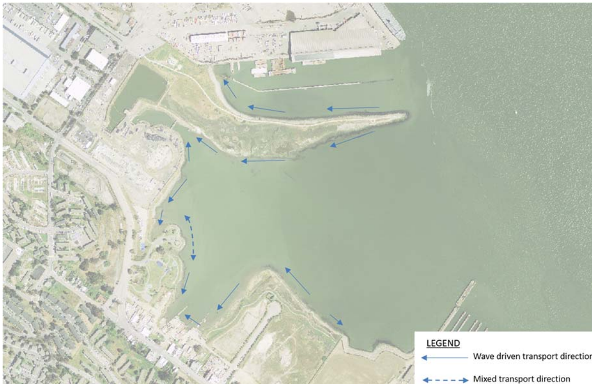
Figure 29: Overall Wave Driven Sediment Transport Patterns
