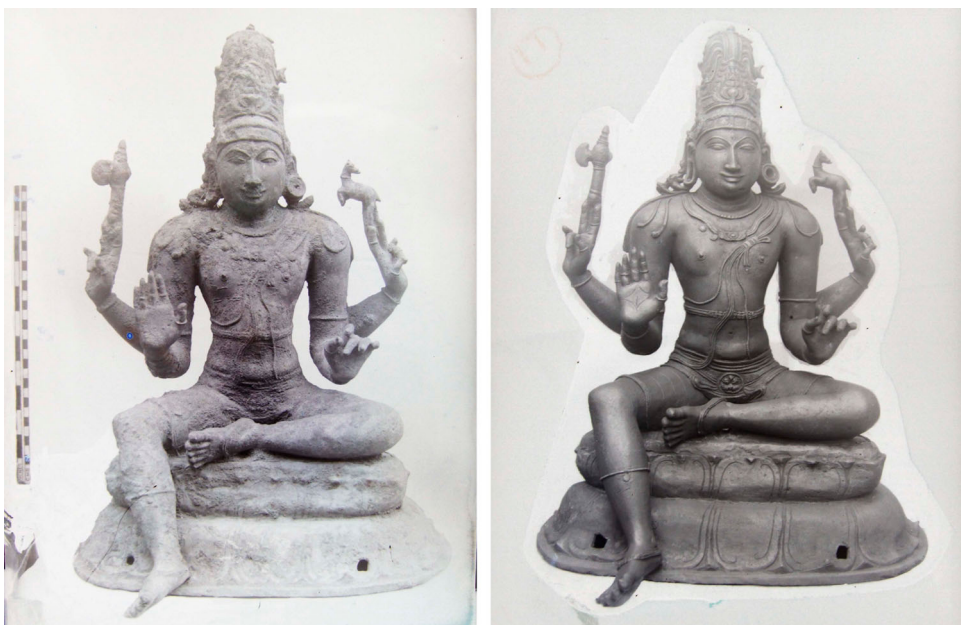
Figure 4. A bronze image before (left) and after (right) electrolytic reduction. Image courtesy of the Government Museum, Chennai.
