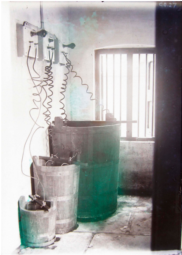
Figure 1. View of the wooden barrels first used as electrolytic reduction tanks. Image courtesy of the Government Museum, Chennai.
