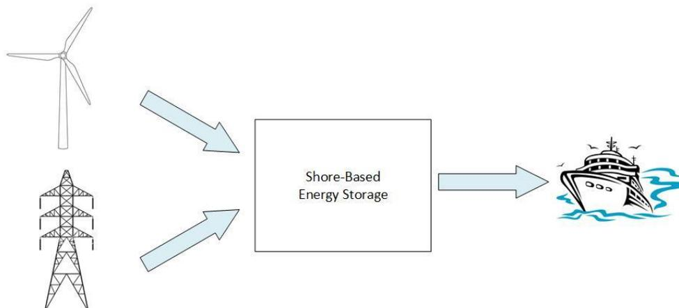
Finally, an energy storage resource dockside could allow for operations to continue in the event of a power outage affecting the terminal area or a wider geographical area. The number of voyages possible would be dependent on the size of the shore-based energy reserve.
