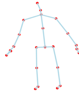
Figure 1 The red dots are joints tracked by the Kinect sensor.
