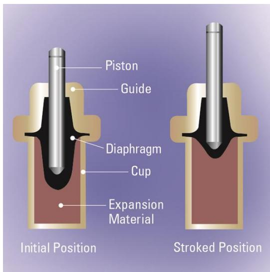
The temperature within a mixing valve is affected by fluctuations in the inlet water temperature and pressure. Heat is transferred through the walls of the sensor and passed to the media. In the example in Figure 2, that media is paraffin. Ether can also be utilized, and some valve manufacturers use a bimetal coil.<sup>5</sup>
