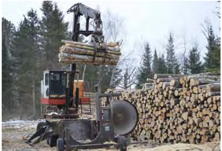
Bill Stangler works on the landing, operating the company's loader/slasher.
