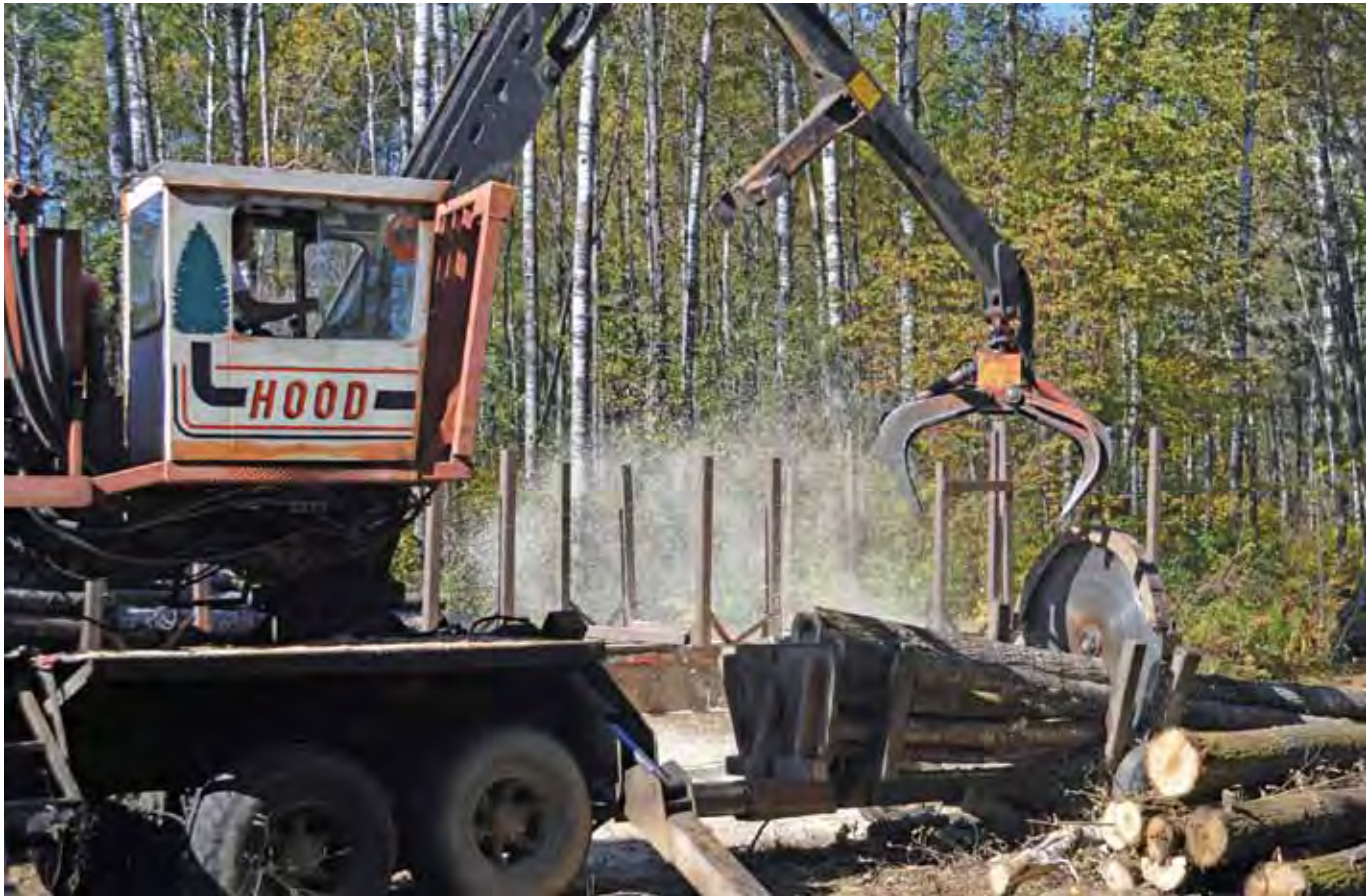
Scott Broberg slashes aspen with a Hood 12,000 slasher loader, featuring a 60 inch saw.
