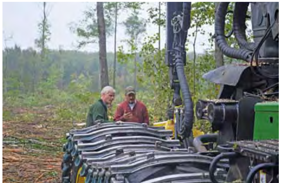
Pittack shows Thissen the harvesting head on his cut-to-length processor.
