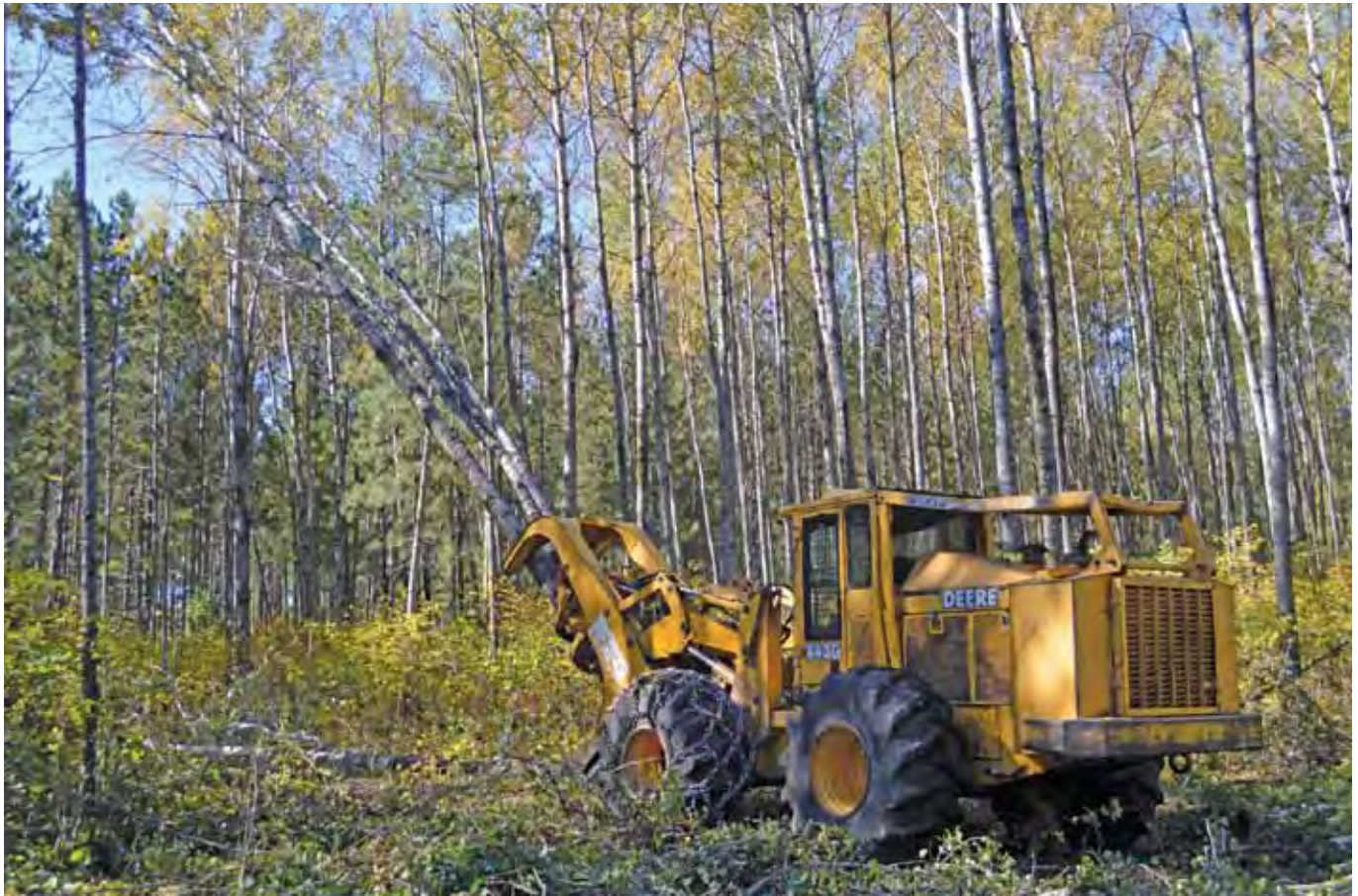
Ron Guertin operates a John Deere 843G feller buncher to harvest aspen on an Aitkin County sale near Jacobson.
