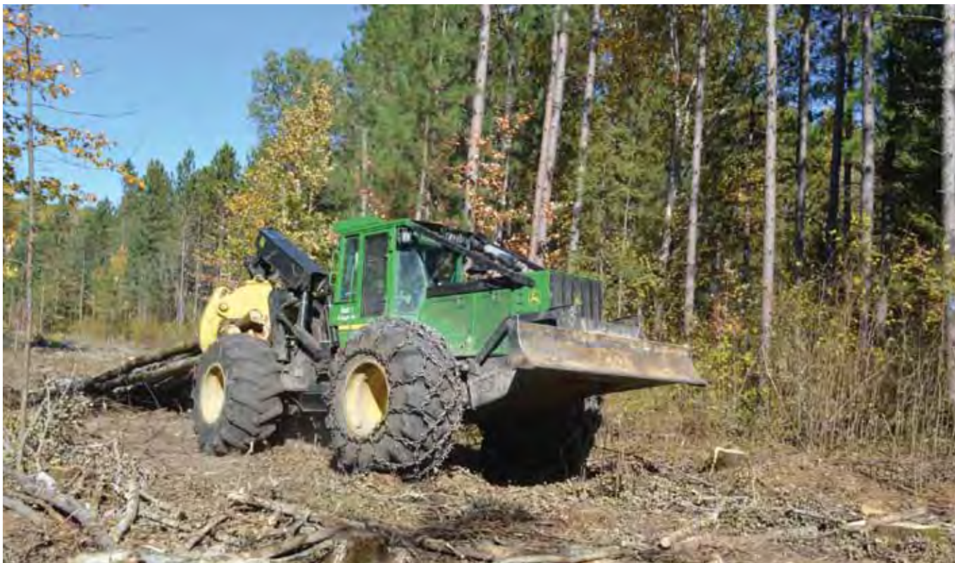
Guertin drags wood to the landing with a John Deere 648H skidder.
