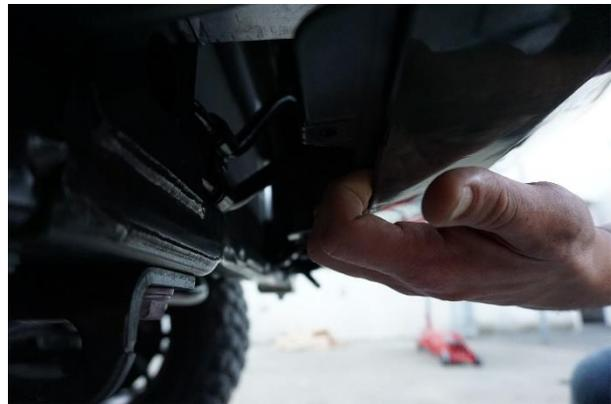
3. Remove plastic Crash Bar Cover (i), Front Cross Bar Bolts/Factory Tow Hook (ii), and Aluminum Crash Bar (iii). Save the nuts, these will be reinstalled.
