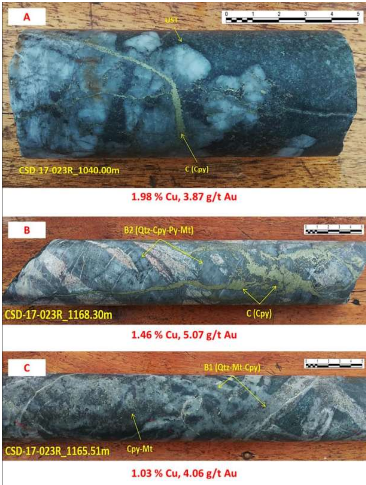
Figure 3: Selected examples of high grade mineralisation encountered in Hole 23R, UST crystals in the parent porphyry melt (A), intense chalcopyrite flooding (B), and intense chalcopyrite-magnetite mineralisation.
